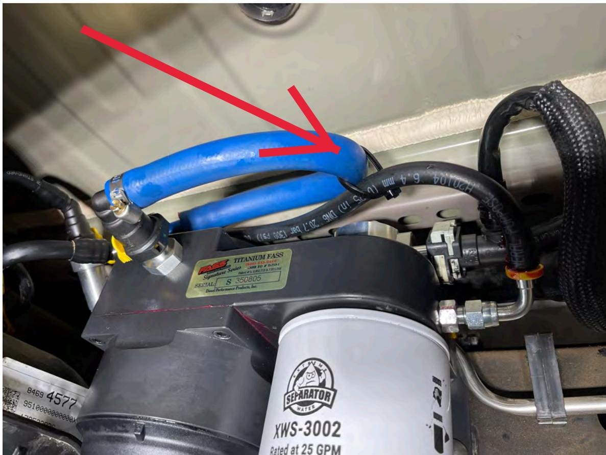
T. Apply grease to the XWS-3002 gasket, then install onto the FASS System.
