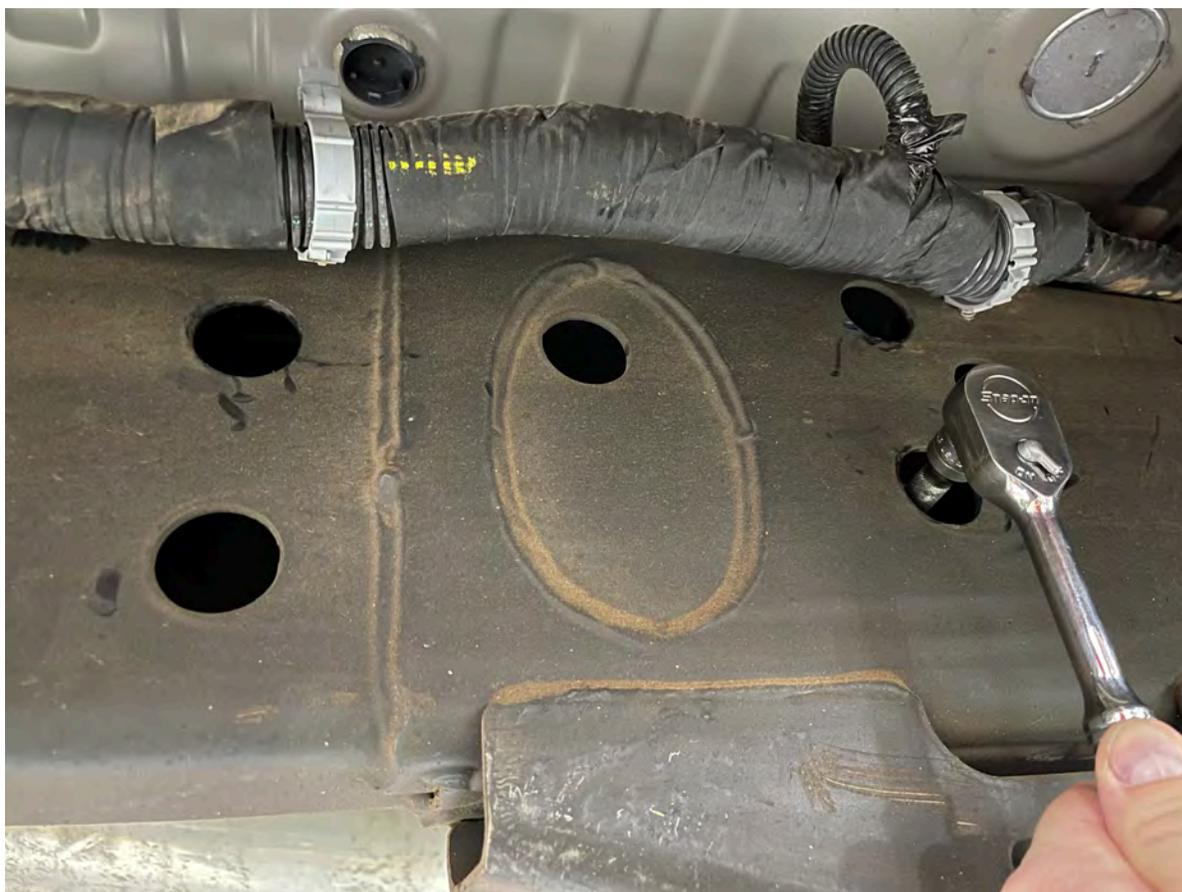
**D. Using a 13mm ratchet wrench, remove the two bolts securing the filter housing to its bracket. It may be necessary to partially pull the bracket away from the frame to remove both of the bolts. Remove the OEM filter housing and bracket from the truck.**
