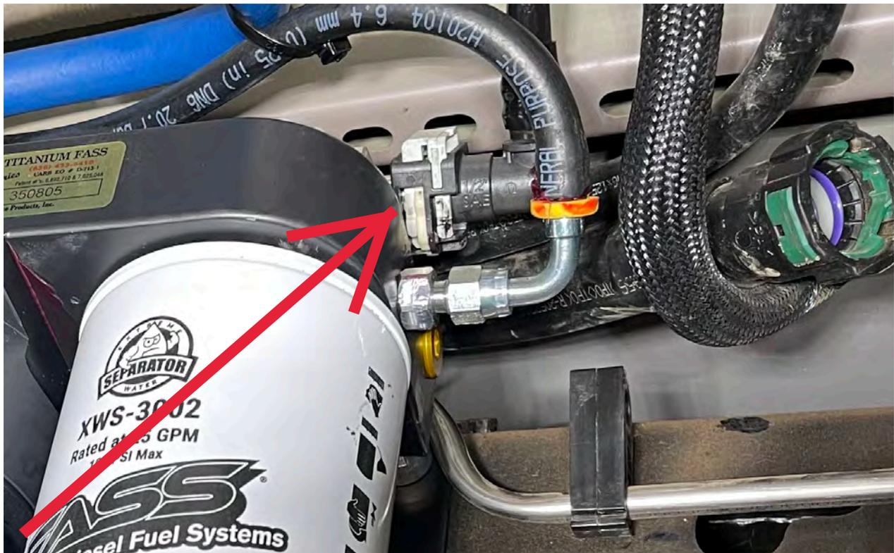
**P. Using grease, install FL-1010 onto PL-2001. Install PL-2001 onto the FASS and tighten accordingly.**
