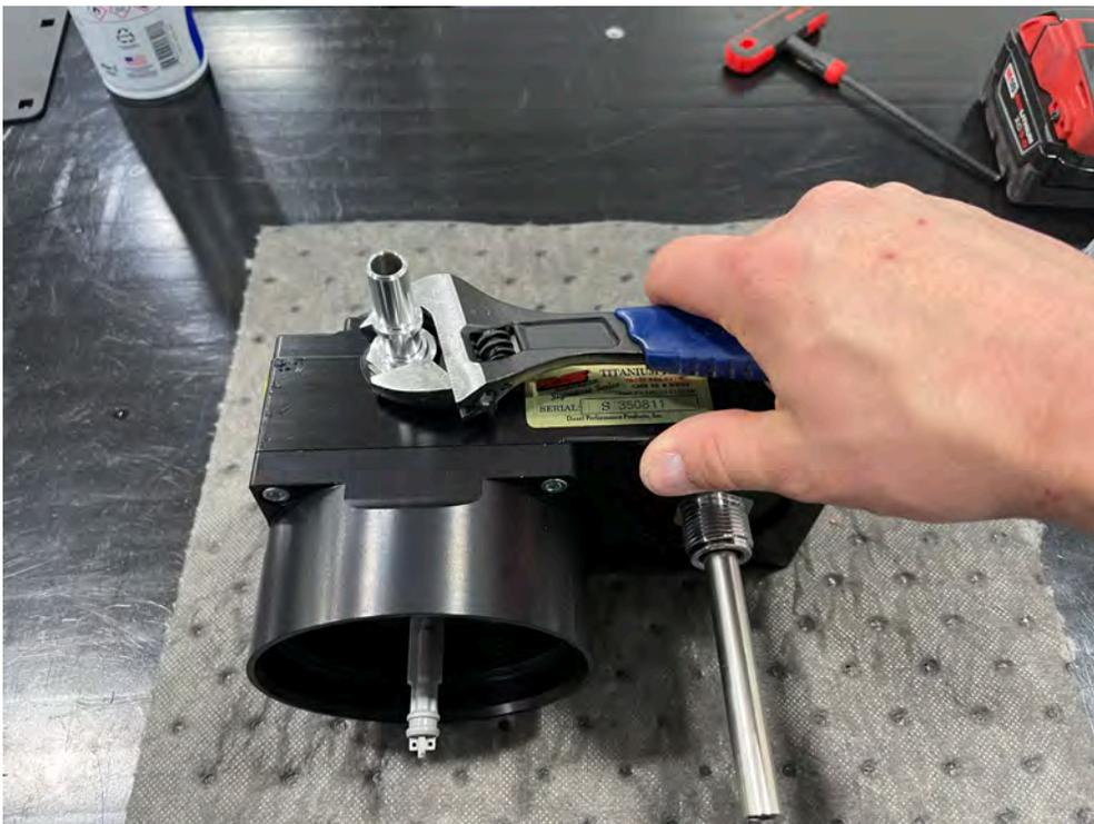
I. Place the two 8mm countersink bolts through L5P-FB-2020 with the two supplied aluminum spacers. Be sure the spacer countersink is faced toward the bolt. Place the bracket onto the FASS and tighten accordingly.
