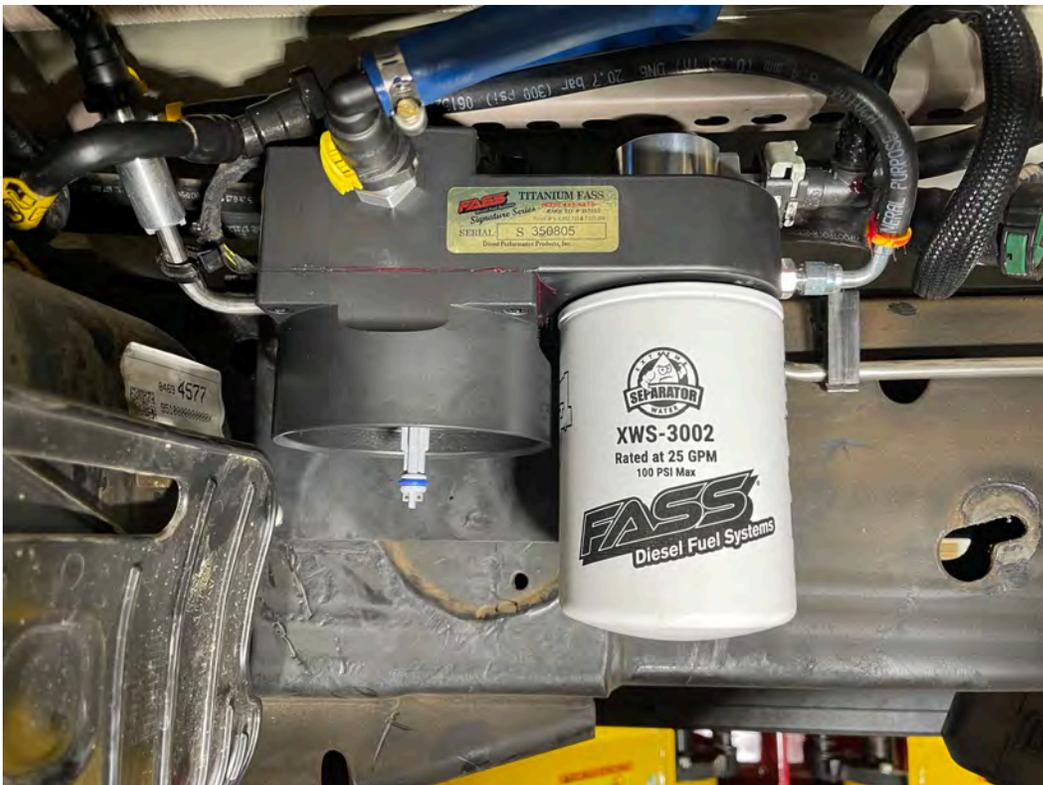
**U. Install a new filter into the OEM fuel filter cap, then thread the cap into the FASS System. Tighten accordingly.**
