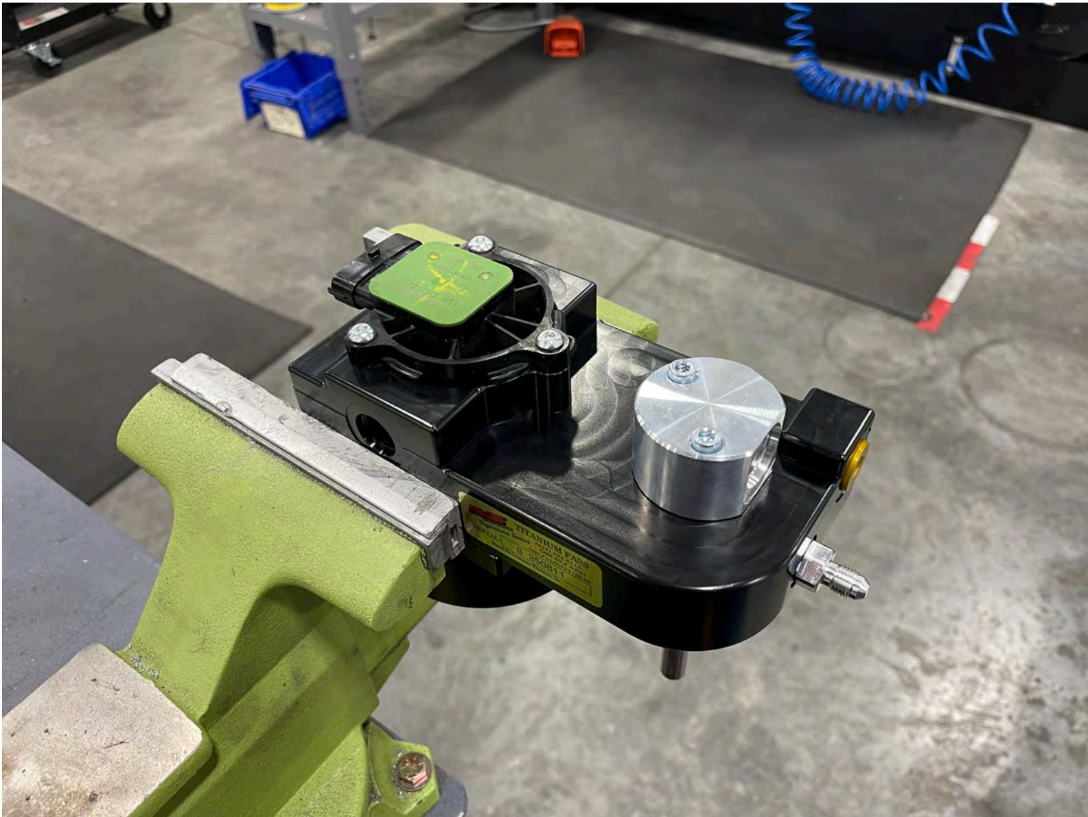
**H. Install 10-ORB-500-QC into the fuel manifold and 8-ORB-500-QC into the open port on the side of the filter base. Tighten both fittings accordingly.**
