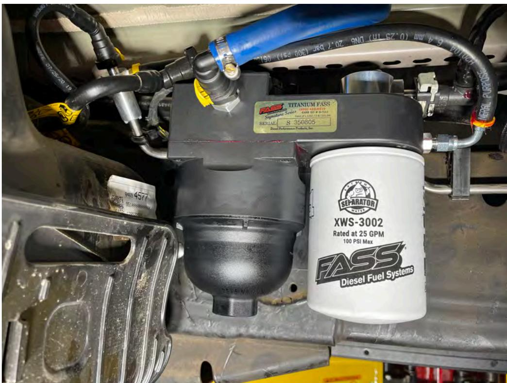
**V. Prime the fuel system, start the truck, and check for fuel leaks.**
