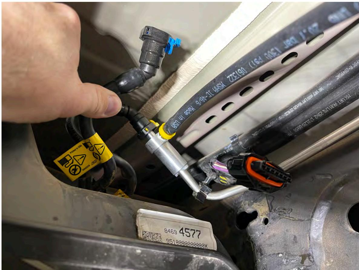
**NOTE: THE OEM FILTER SECTION IS REMOVED FROM THE FASS IN THE BELOW PICTURE FOR VISABILITY PURPOSES.**
