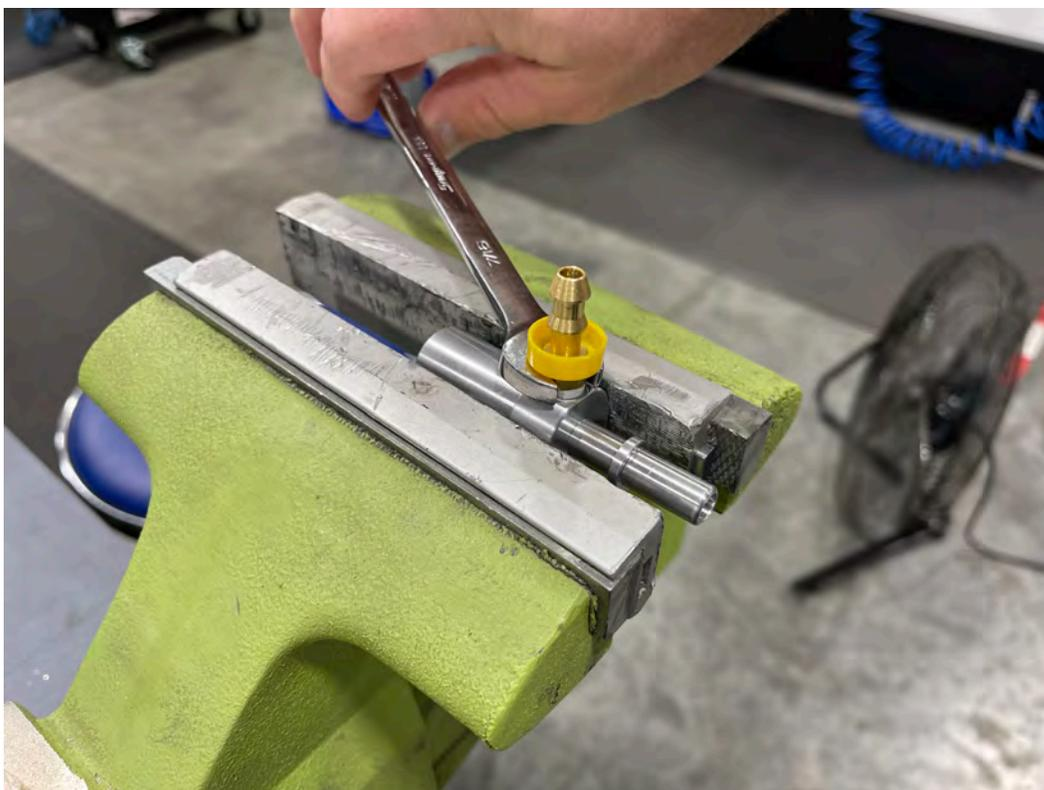
L. Using grease, place FL-1010 onto PL-1011.
