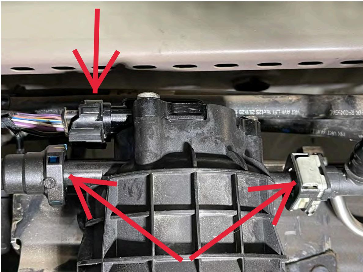
**C. Loosen the three nuts securing the filter housing bracket to the frame, it is not necessary to completely remove the 3 nuts.**
