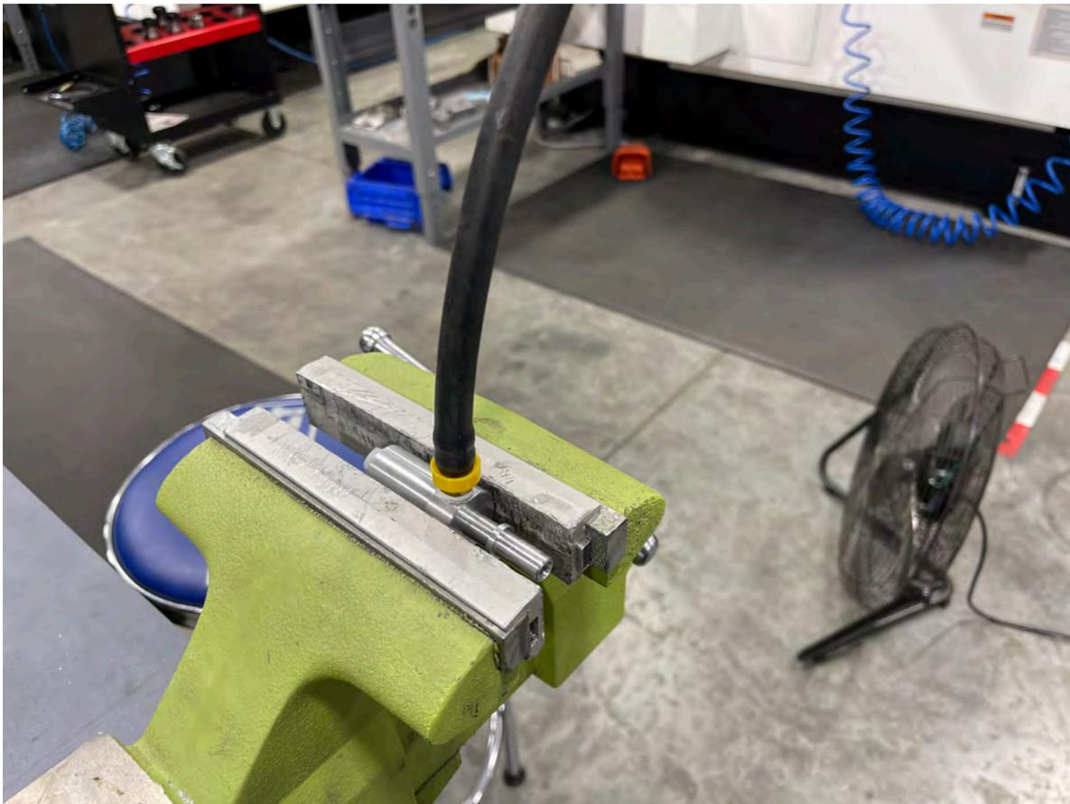
**M. Install 375-QC-1E-NPT onto the fuel return line as shown. Be sure the locking clip is fully seated on the fuel line after it is installed!**
