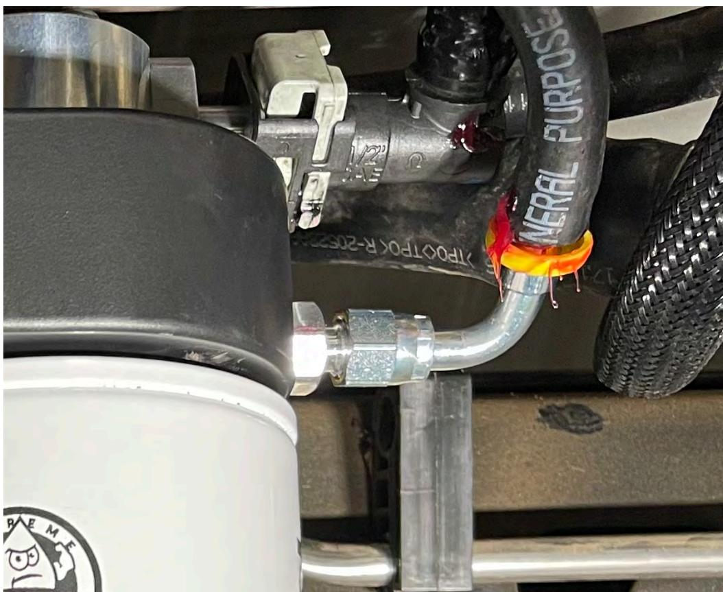
**Q. Using grease, install PL-1212 into one end of FL-1002 and install A624C56-55-05 into the opposing end. Install hose clamp HC-1001 onto the the end with A624C56-55-05 and tighten accordingly.**
